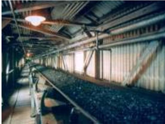
The rollers of conveyor belts can heat up and ignite the coal dust
